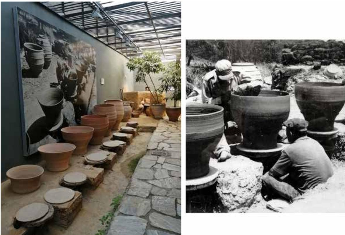
Fig. 20. Hand-operated wheels below the ground for the manufacture of Cretan *pithoi* (Centre of the Study of Modern Ceramics, Athens, Greece).
